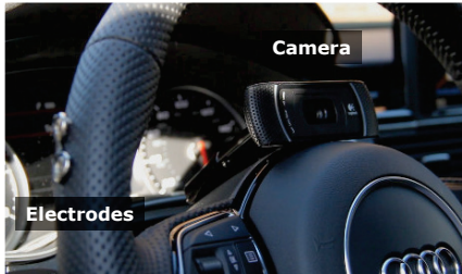
Figure 1. Close-up of the steering wheel showing the camera (center) and the electrodes (left) to comfortably monitor physiological signals.
