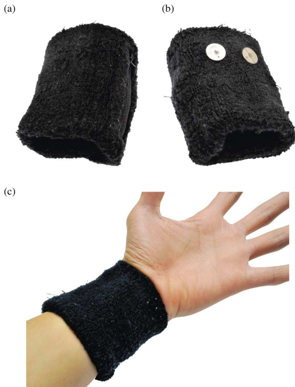
Fig. 3. Wearable EDA sensor. (a) Final packaging in an attractive and inconspicuous wristband. (b) Disposable Ag/AgCl electrodes attached to the underside of the wristband. (c) Wearable EDA sensor can be worn comfortably on the wrist for long periods of time and during daily activities.
