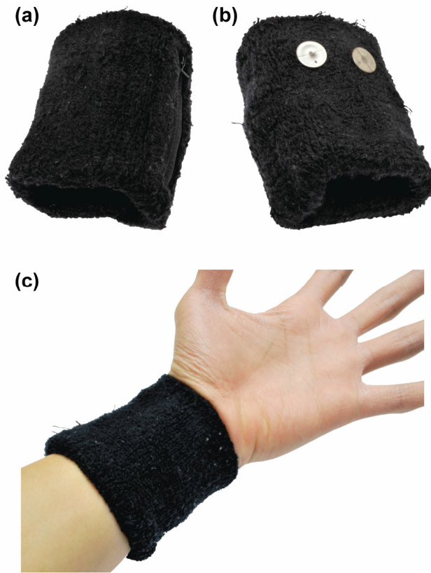
Fig. 1. Wearable EDA sensor. (a) Sensor is inside stretchy breathable wristband. (b) Disposable Ag/AgCl electrodes attached to the underside of the wristband. (c) The EDA sensor can be worn comfortably for long periods of time.
