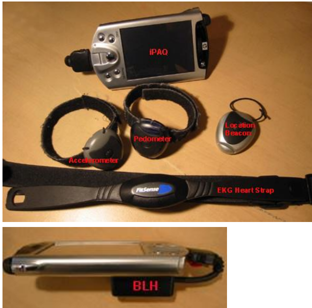
Figure 1. Custom hardware for the PMobile System: Top: iPAQ with sensors. Bottom: iPAQ with attached Body Lan Hub (BLH), which communicates wirelessly to all the sensors.
