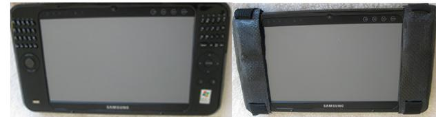
**figure 2:** The Ultramobile's keyboard (left) and our fabricated external shields (right).
