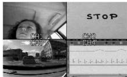
Fig. 2. A sample frame from the quad split video collected during the experiment. The upper left panel shows the driver facial expression, collected from a camera mounted on the steering column. The upper right panel shows the camera used for experimenter annotations where a “stop” annotation is shown. The lower left panel shows road conditions and the lower right panel shows a visual trace of the physiological signals as they were being recorded.
