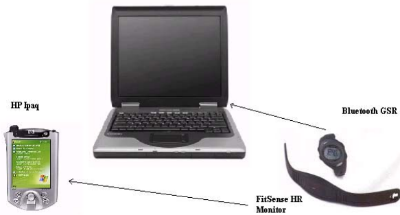
Figure 1: INNER-active Journal System. FitSense Heart Strap sends data to iPAQ while Bluetooth skin conductivity sensor sends data to laptop.
