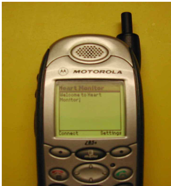
Figure 4: The Motorola iDEN phone, i85, which provides the main display and off-body communication and support functions.
