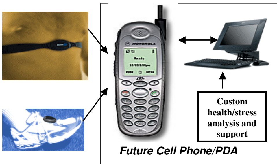
Figure 3: The FitSense chest-strap and foot pod communicate via Motohub to the Motorola iDEN phone, which communicates to an off-body workstation. The workstation can analyze data, make comparisons, and in the future, deliver conversational feedback to support the wearer, or notify medical personnel of the wearer's situation.
