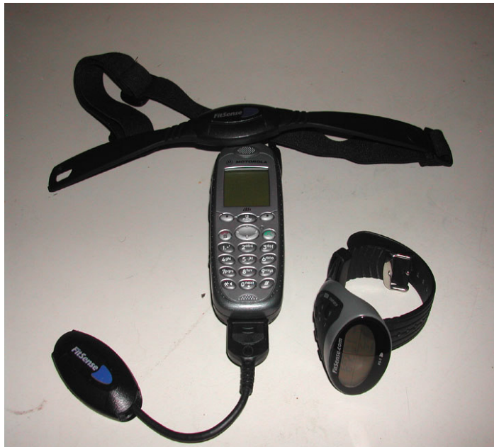
Figure 2: The Motorola iDEN phone and FitSense chest strap, Motohub, and wristwatch.
